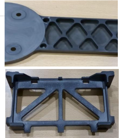
Complex shaped sintered SiC parts for aerospace applications
